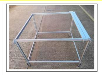
Place the remaining Support Beam and the 3 x Standard Beams over the brackets (DO NOT TIGHTEN THE GRUB SCREWS AT THIS POINT) then place the remaining end frame over the Beams (this may be easier with help from an assistant).
